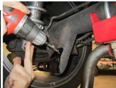
Figure 3 – Drilling for 3/8" reinforcement
