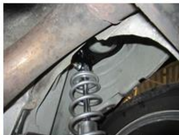
Fig 5 – Upper bracket install
